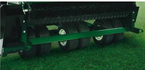
Turfco's Mete-R-Matic III and XL topdressers utilize the same patented ground-drive system. When you speed up, slow down or cross uneven terrain, the conveyor belt and brush automatically adjust at the same rate to provide a consistent and even application every single time. No hydraulics, no pumps and no engines. Just hook up and go.
