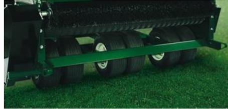
Turfc's Mete-R-Matic III and XL topdressers utilize the same patented ground-drive system. When you speed up, slow down or cross uneven terrain, the conveyor belt and brush automatically adjust at the same rate to provide a consistent and even application every single time. No hydraulics, no pumps and no engines. Just hook up and go.
